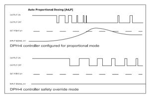
for a fully dynamic dosing control, which adapts for widely varying conditions in a cooling tower or other plant installations. Dosing for an excessive period of time without a corresponding movement in mV is recognized
