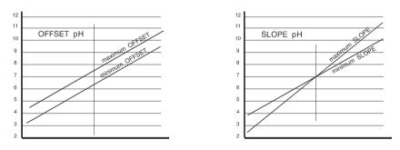
FIG. 5 THE DIFFERENT EFFECTS OF OFFSET AND SLOPE.
