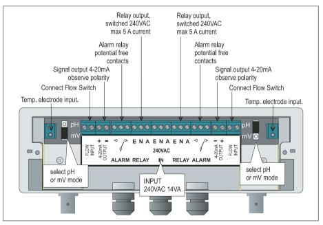
FIG 4 Terminal layout for the DPH-4
