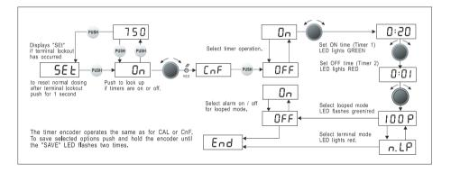
FIG 11 Configuration of Timers.
