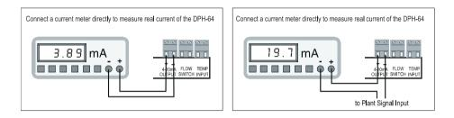
FIG 10 Calibrating 4-20mA with a multimeter.
