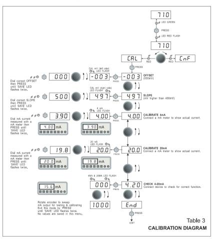
A slope calibration can be performed if the pH is lower than 5.5. or higher than 8.5 or in mV mode between 280mV and 900mV. The message ' **Err** ' will show if this condition is not met. If this is the case PUSH twice, adjust pH / mV for correct value and repeat mV calibration.
