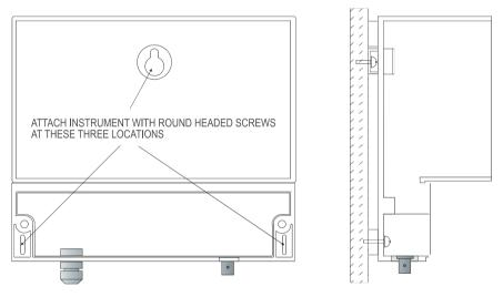
FIG 3 Attaching the DPH-4 to a wall
