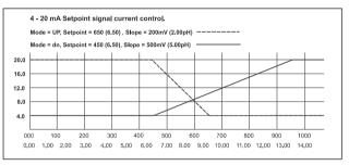
FIG. 9 4-20mA Setpoint Signal current control.
